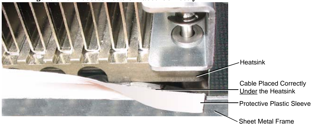
Figure 6-16 Processor Cable Placed Correctly
